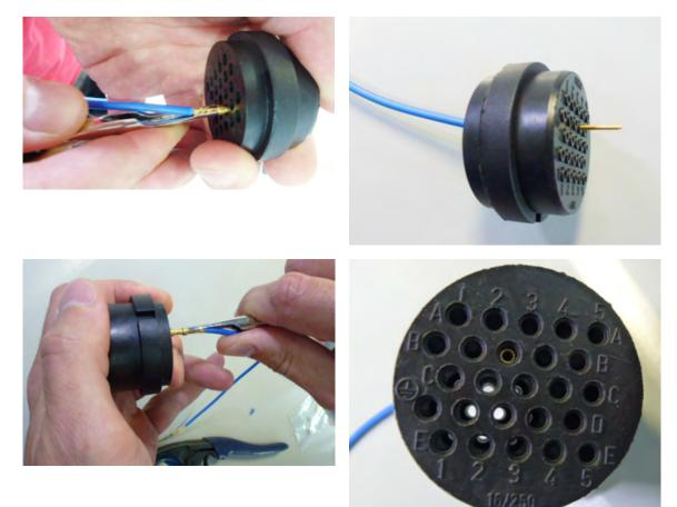
Pins and sockets that are inserted too far are to be pushed back to their engaging point with a removal tool.
