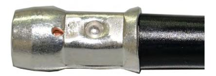
Not correctly crimped. Pay attention to the correct size of the crimping tool.
