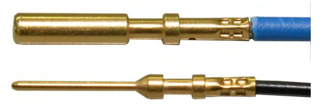
Not correctly crimped.
