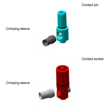
Insert the crimping sleeve into the contact pin or socket and secure using a screw.
