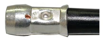
Not correctly crimped.
