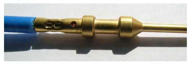
Not correctly crimped.
