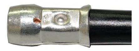
Not correctly crimped. Pay attention to the correct size of the crimping tool.
