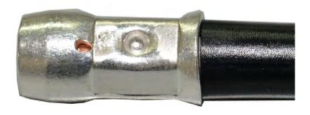
Not correctly crimped.
