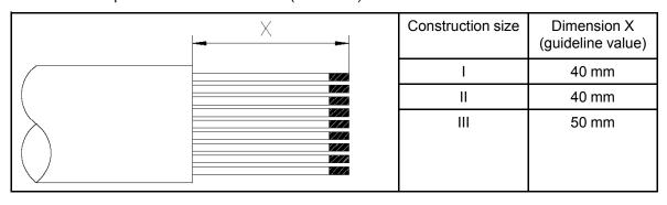
Then strip the individual wires with a suitable tool.
