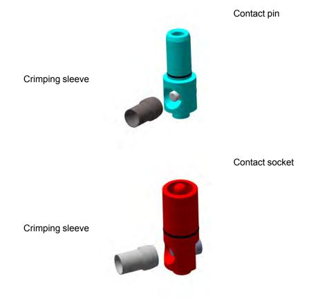
Insert the crimping sleeve into the contact pin or socket and secure using a screw.
