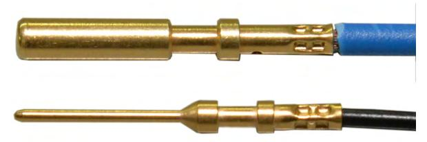
Not correctly crimped.
