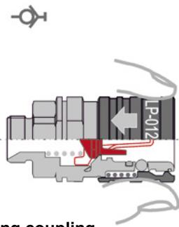
-0- Self-sealing coupling = coupling with valve
