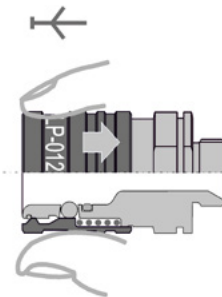
-4- Thru-type coupling = coupling without valve
